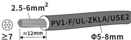
2. Route the stripped cable all the way into the DC connector. Ensure that
