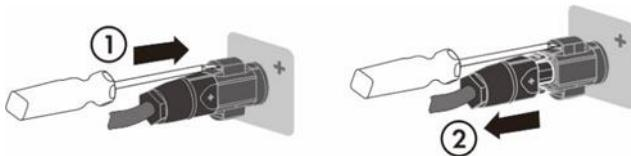
5. Release and disconnect the AC connector. Rotate the socket element counterclockwise to open.
