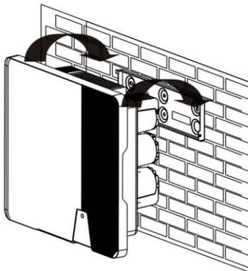
4. Check both sides of the outer fin of the inverter to ensure that it is securely in place.
